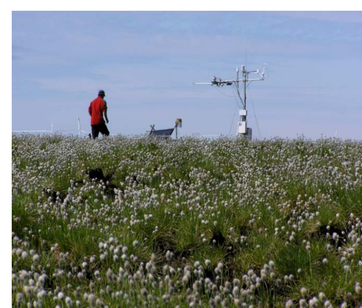
Figure 2. An eddy flux tower in a field of flowering Eriophorum tussocks, North Slope, Alaska.
